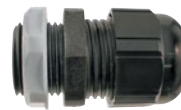
PG12 GROMMET 4GA 7/8" Mounting hole 4GA waterproof firewall bushing Watertight seal when power wires pass through metal Locks securely as bushing is tightened
