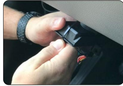
4. For the Nut and Bolt style mounting system: Place the left ear of the connector over the left factory stud and replace and tighten the 8mm nut removed in step 1. Secure the right ear of the connector to the under dash using the included self tapping screw (Fig. C).
