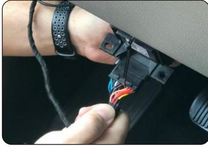
3. Secure the OBD II connector and the harness together using one of the included wire ties and cut off any excess wire tie that is not needed (Fig. B).
