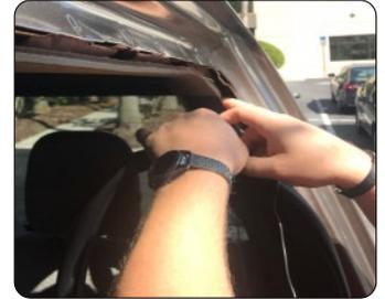
13. Clean and dry mounting location with an alcohol pad prior to mounting camera. Mount the camera on the rear window using the supplied adhesive on the camera. Keep in mind to not mount camera in a location that will interfere with rear view mirror visibility. Connecting to the dash cam using the Thinkware smartphone app may be necessary to verify that the picture is right side up and the entire rear of vehicle is in the frame. See Fig. E and F for clarification.
