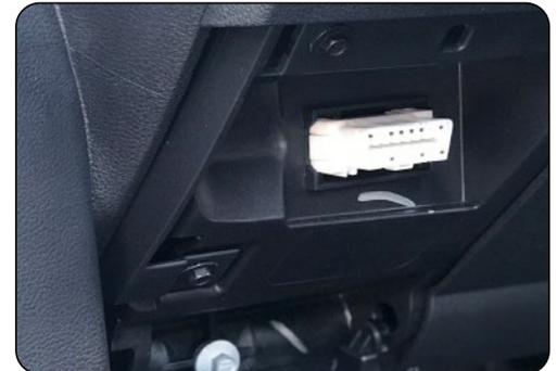
2. Connect the male end of the included Plug-n-Play HWK-TW01-HAR to the vehicles factory ODB II connector (Fig. A).
