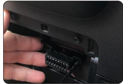
5. Remove the A-Pillar trim panel; this may require the removal of 2 x 10mm bolts. Route the Thinkware power cable over to the driver side of the vehicle, up the A-Pillar (Fig. E) and across the front of the headliner (Fig. F & G) so that it exits the headliner at the factory notch above the rearview mirror. **NOTE: When routing cables near the side curtain airbag, be sure to route them in a way that will not impact the airbags' ability to deploy in the event of an accident.**
