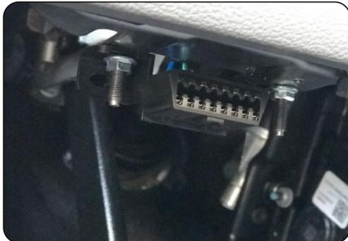
1. Locate the OBD II connector in the vehicle and release it from the mounting surface. This may require the removal of two 7 or 8mm nuts from the studs securing it to the under dash (Fig. A) or by depressing the two side clips, with a plastic dash trim tool, securing it behind the drop down plastic cover (Fig. B).
